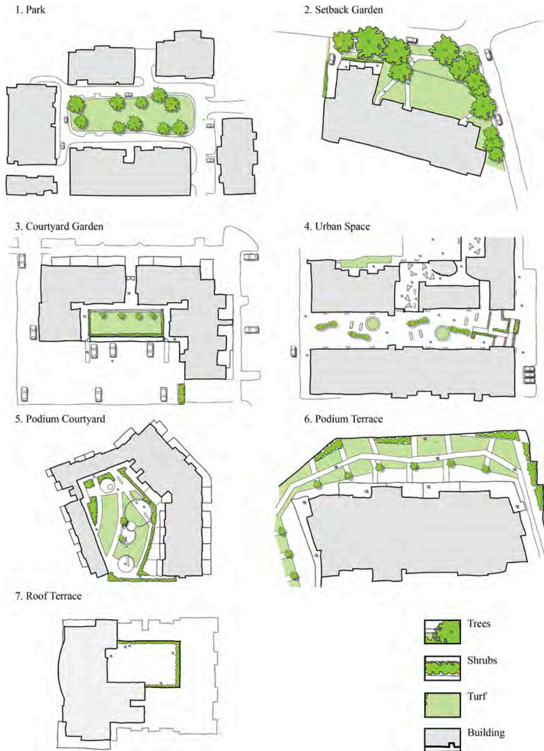
Fig. 1. The COS typology. These plans are indicative only as our ethics approval prevents the release data identifying the study buildings.
