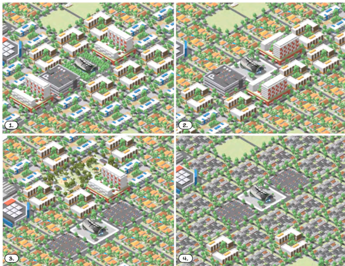
Fig. 2. A comparative image of the urban densification strategies: 1. TOD Pedestrian Pockets: Urban densification around a train station, 2. TOD Transit Boulevards: Urban densification along a major road, 3. Greenspace-Oriented Development (GOD): Urban densification around parks, and 4. Hidden density: Urban densification in backyards.
