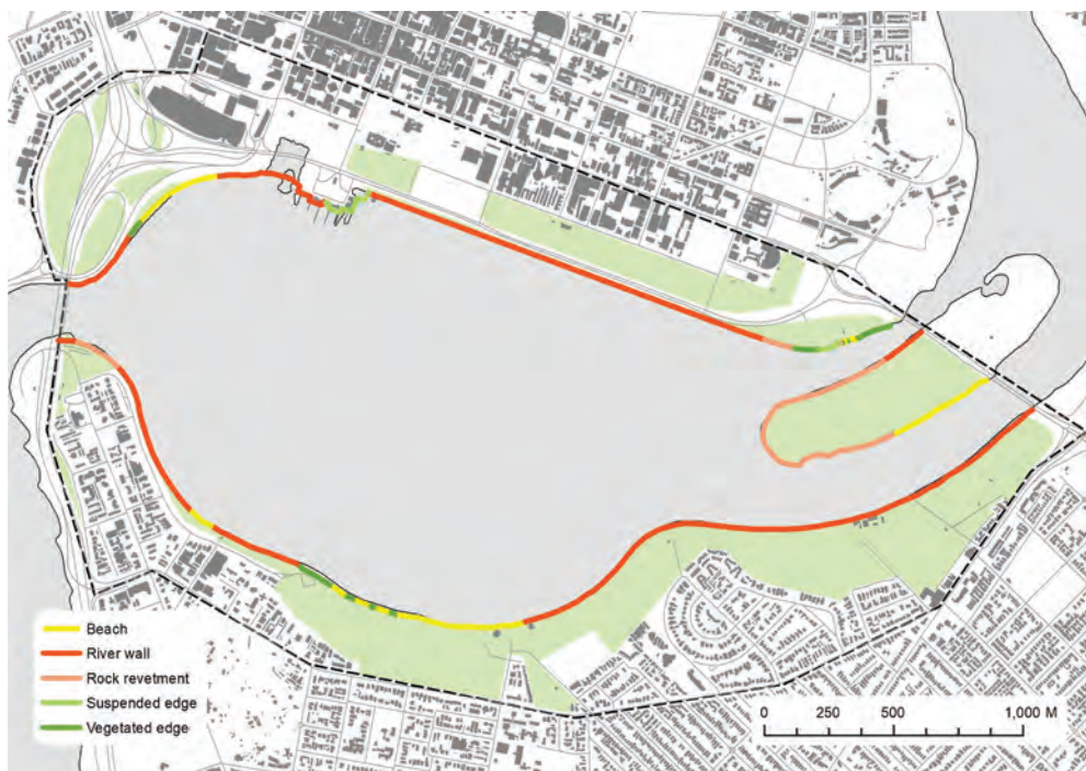
Figure 2. Perth water edge types plan. Fortified sea walls and embankments are the predominate edge condition.
