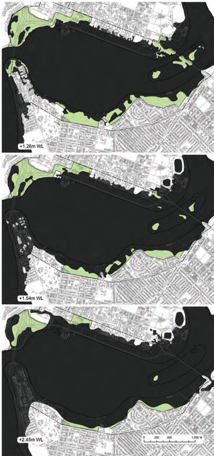
Figure 6. Predicted water levels (WLs) and implications for the CPRP system. The 1.26 m WL relates to 0.56 m SLR plus a 0.7 m high tide, and the 1.54 m WL relates to 0.84 m SLR plus a 0.7 m high tide. Also included is a low-likelihood layer of 2.45 m WL (1.75 m SLR plus a 0.7 m high tide) which factors in ice-sheet instability under for Shared Socioeconomic pathways 8.5. Water levels shown are indicative only.
