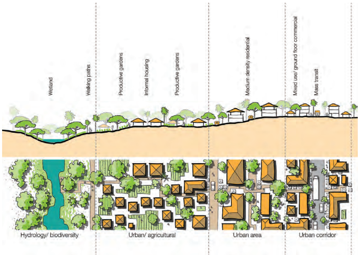
Figure 12. Corridor development on elevated land provides residents with easy access to public transport and economic opportunities and preserves Gulu’s extensive wetland systems, which deliver flood mitigation and water quality benefits, as well as public open space. Figure adapted from the New Urbanist transect diagram. Note, this figure is indicative only. Figure by the authors.
