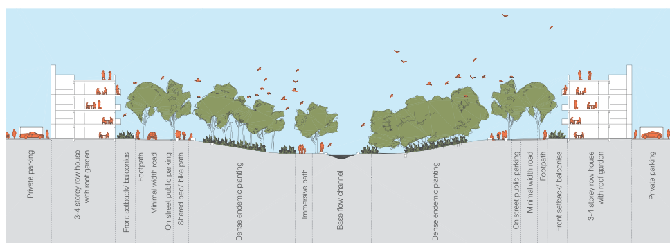
Figure 13. Binding the Living Streams and adjacent streets into a single composition. Streets running adjacent to the Living Stream should be one-way or two-way (of a minimal width) and planted with street trees in such a way that binds them into the Living Stream as one 'single composition'. This perception can also be increased by grading the adjacent streams so that they 'fall' towards the Living Stream, and have flush kerbs, all of which helps to unify the adjacent streets and the Living Stream visually and hydrologically.
